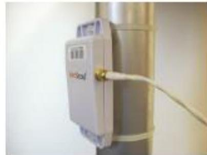
*Tag mounted on a pole using tie wraps*
