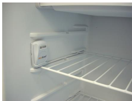
Tag attached by a cradle taped to a fridge wall
