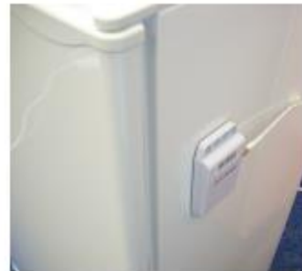
Tag mounted on a refrigerator using velcro
