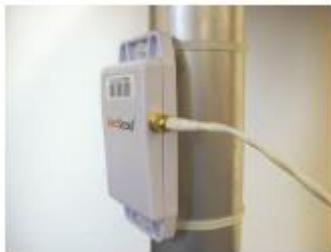
Tag mounted on a pole using tie wraps
