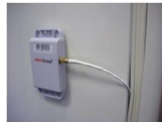
Sensor inserted through refrigerator door
