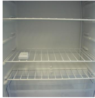
Tag attached by cradle strapped to the fridge's net
