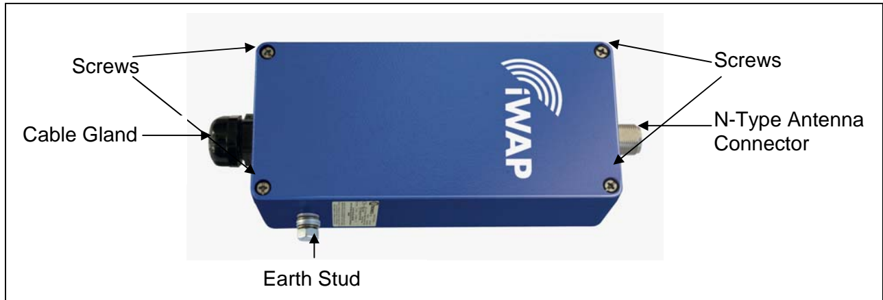
Figure 1 iWAP400 outer view showing connections
