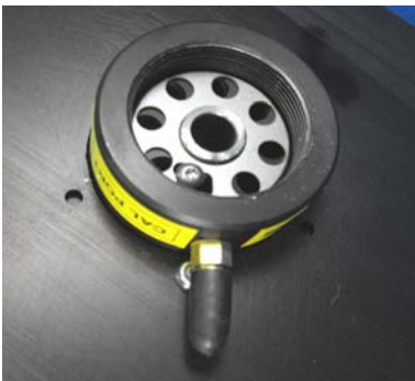
Multiple orifice exits to increase homogenisation of sample
